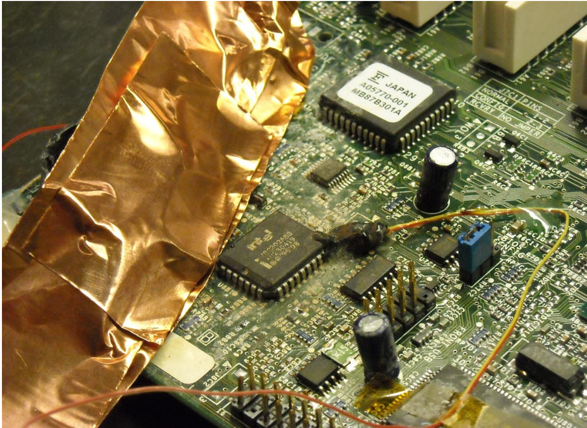
Figure #8 - After repeated heating, the copper also became discolored. This did not affect performance
