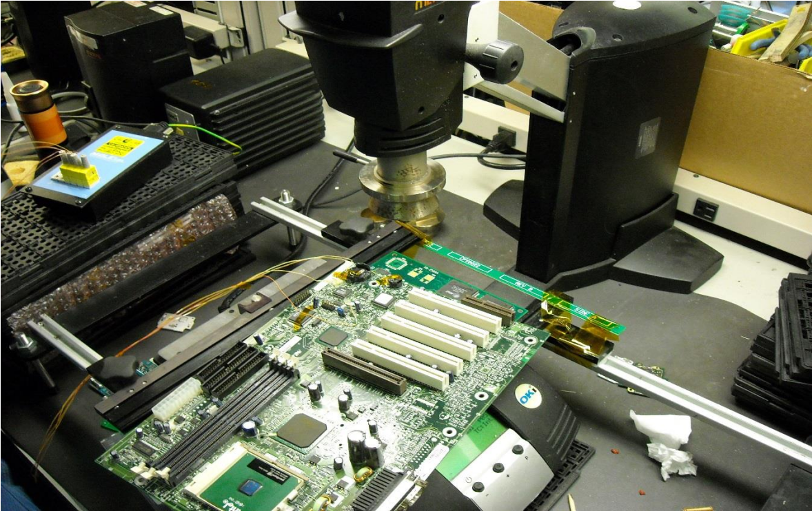
Figure #3 - The board was first placed on a board holder as part of the Metcal QX-2 hot air system used for the trials. Kapton™ tape was used to hold four thermocouples in place until epoxy was added.
